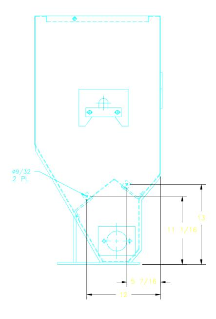
ATTACH HF12-23 AUGER SHIELD TO MOTOR END OF FEEDER. THIS WILL LEAVE THE DISCHARGE END OF THE AUGER OPEN.
